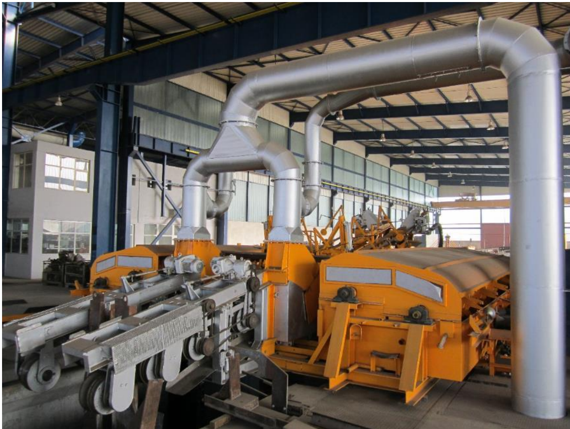
Magnetic rollers and pipe extraction machine
