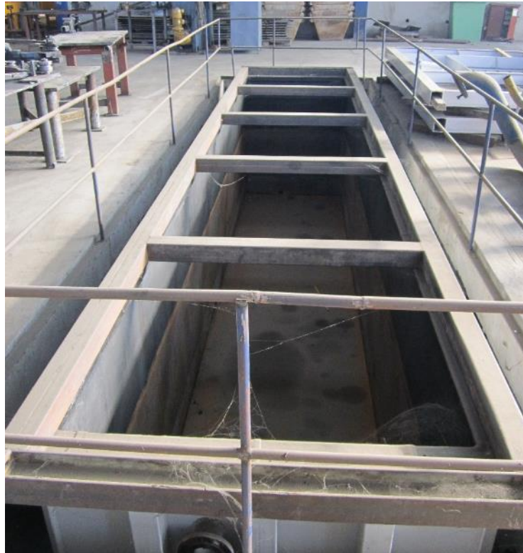
Zinc bath for other constructions
