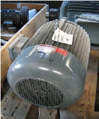
2596 Elektromotor 22/38 kW, 220/380 V, 50/87/120 EMOD FK 200 L / 4 T
