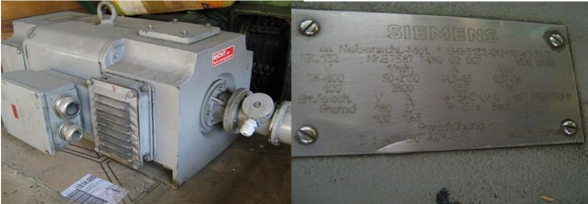
2609 Elektromotor 50/65 kW, 380 V/50 Hz, IP 23 EMOD
