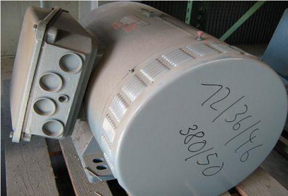
2602 Elektromotor 11/22/32 kW, 380 V / 50 Hz, IP 23
