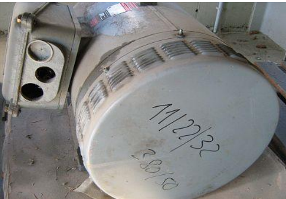
2603 Elektromotor 9/18/28 kW, 380 V/50 Hz, IP 23
