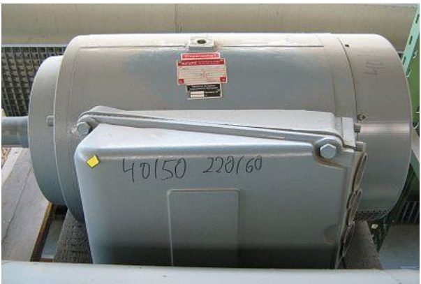
2600 Elektromotor 50/65 kW, 220 V/50 Hz, 181/230 EMOD
