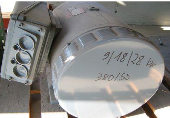
2603 Elektromotor 9/18/28 kW, 380 V/50 Hz, IP 23
