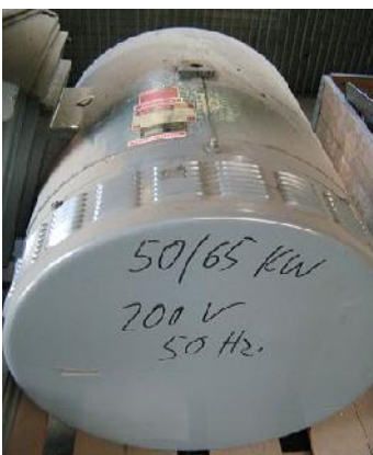
2600 Elektromotor 50/65 kW, 220 V/50 Hz, 181/230 EMOD
