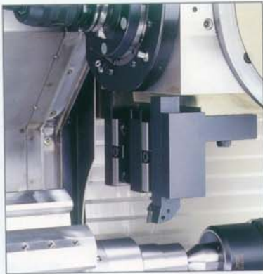
Finishing with the 3rd station (assist station)
